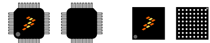
144 LQFP 20 x 20 x 1.6 mm Pitch 0.5 mm 144 BGA 13 x 13 x 1.7 mm Pitch 1 mm
