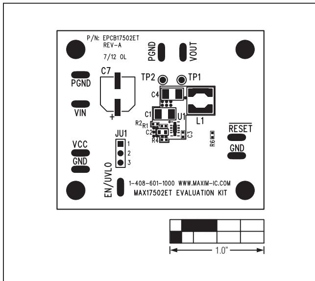
Figure 7. MAX17502E EV Kit Component Placement Guide—Component Side
