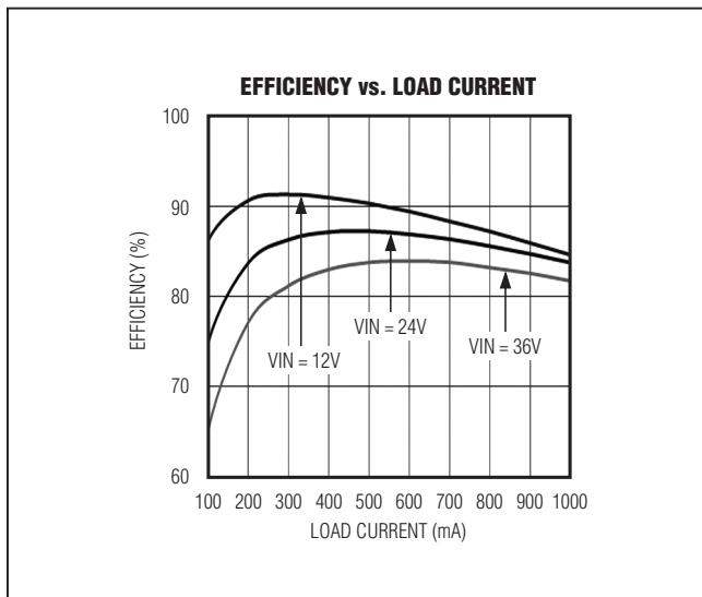
Figure 2. MAX17502E Efficiency
