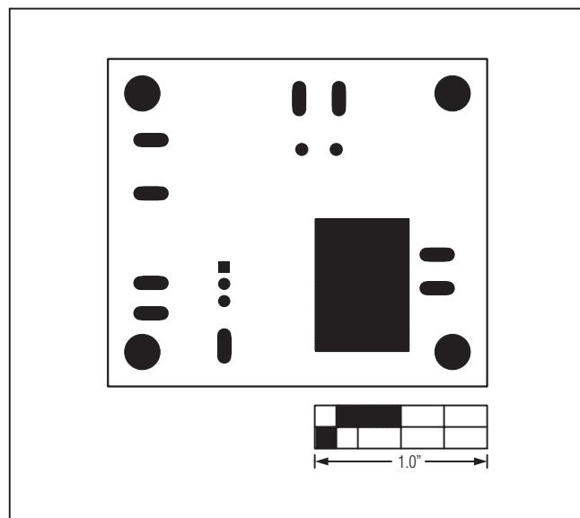
Figure 11. MAX17502E EV Kit PCB Layout—Bottom Solder Mask
