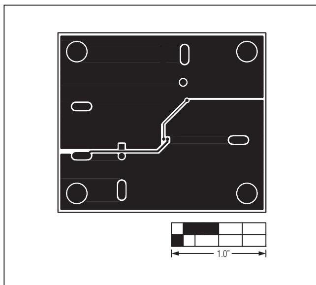
Figure 9. MAX17502E EV Kit PCB Layout—Solder Side
