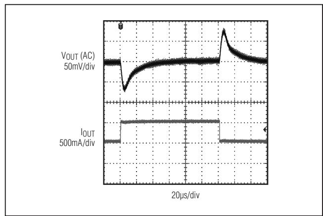
Figure 5. MAX17502E 500mA to 1A Load Transient
