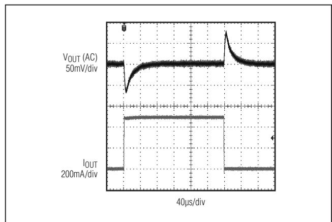
Figure 4. MAX17502E No Load to 500mA Load Transient
