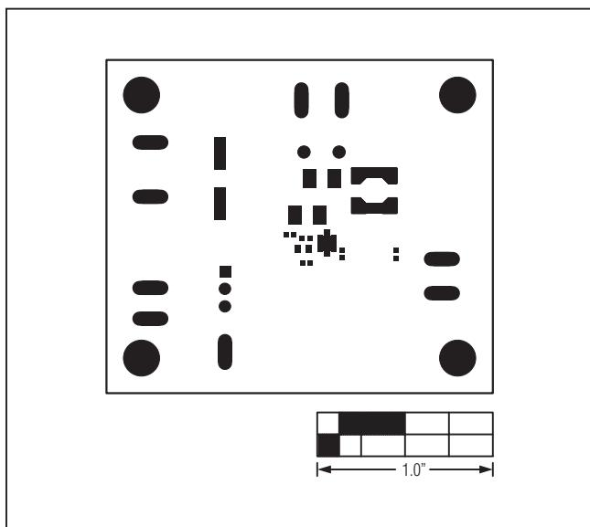
Figure 10. MAX17502E EV Kit PCB Layout—Top Solder Mask
