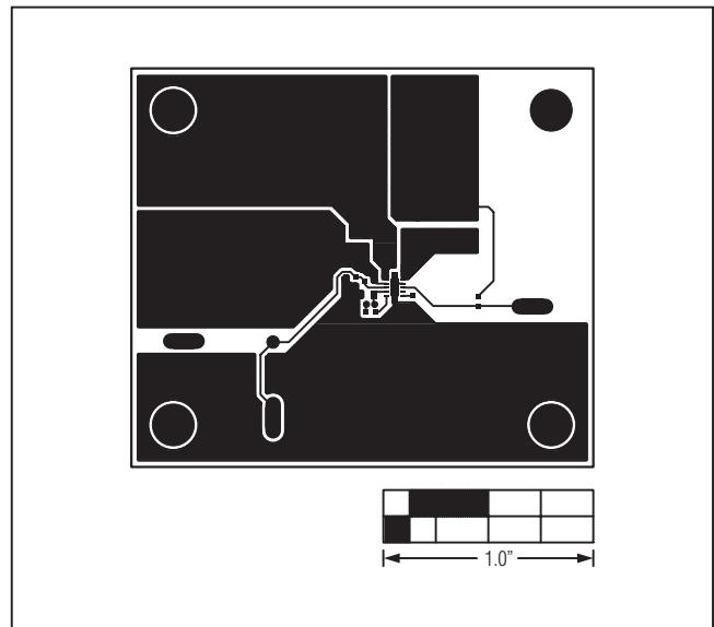
Figure 8. MAX17502E EV Kit PCB Layout—Component Side
