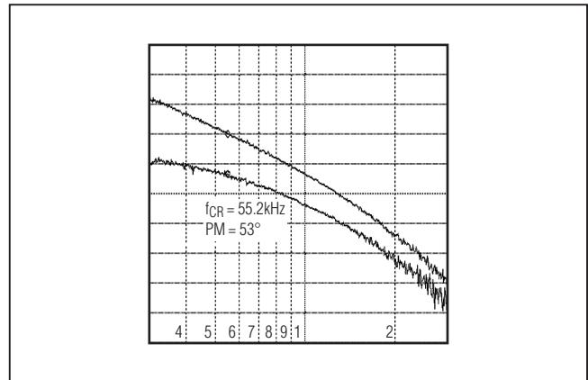
Figure 3. MAX17502E Full-Load Bode Plot (VIN = 24V)
