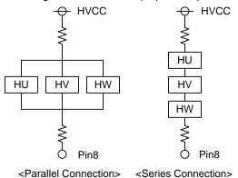
Figure 23. Example of Hall Elements Connection
