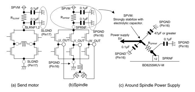
Figure 26. Position of Ceramic Capacitors
