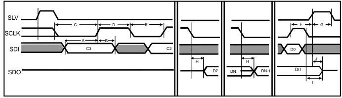
Figure 4. SPI Input / Output Timing
