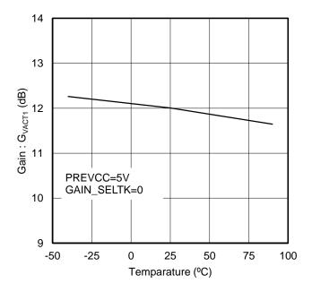
TK Voltage gain 1 (Low gain mode)
