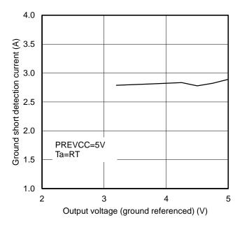
Figure 24. Output voltage vs Ground short detection current
