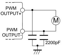
Figure 28. Snubber Circuit
