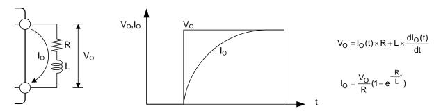
Figure 18. Current Waveform Including Impedance Component
