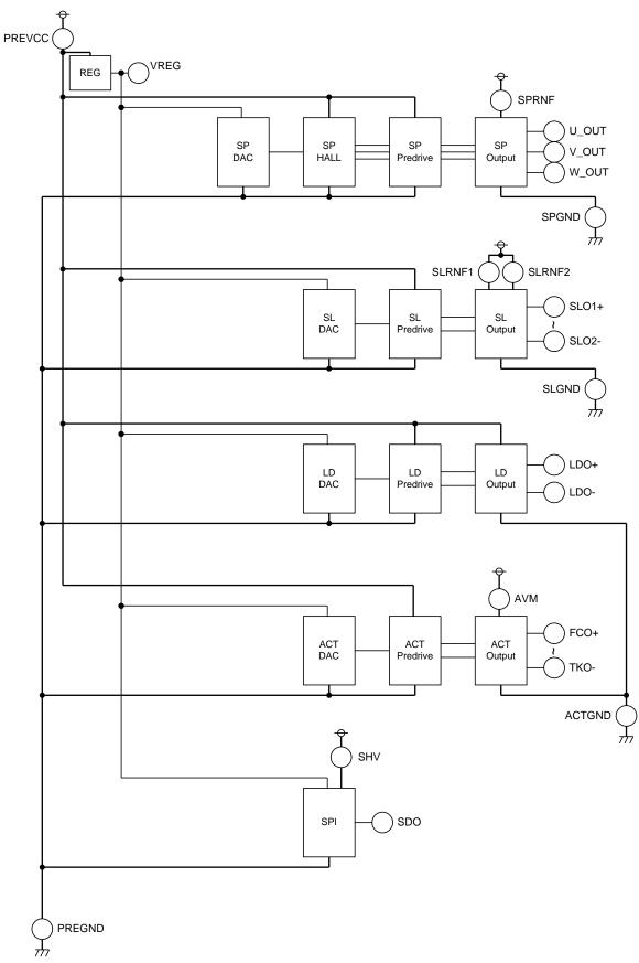
Figure 30. Power Supply and Ground
