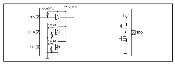
Figure 9. SPI Input / Output Terminal Processing
