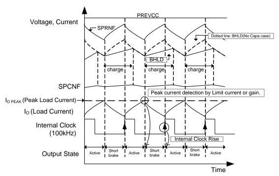
Figure 20. Spindle Driver Operation Timing Chart
