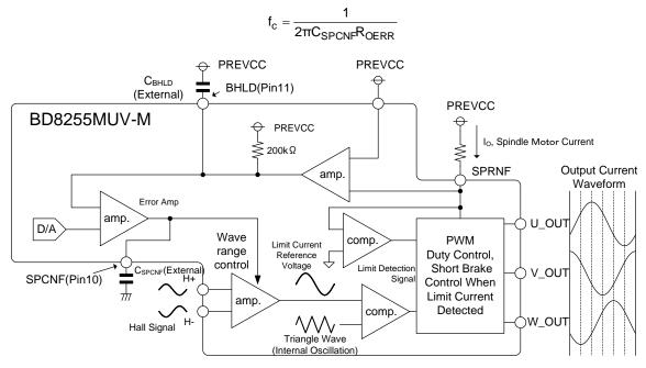
Figure 21. Spindle Driver Block Diagram
