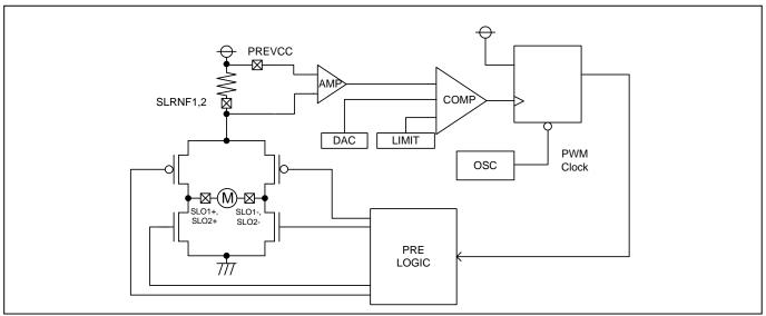
Figure 14. Sled motor driver block
