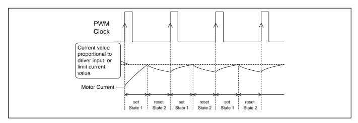
Figure 16. Sled Motor Driver Operation Timing Chart
