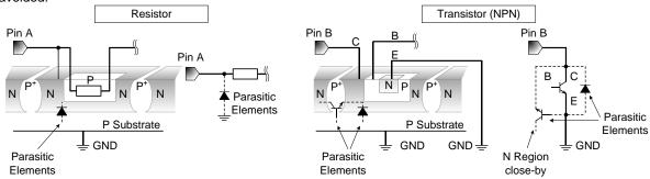
Figure 33. Example of monolithic IC structure
