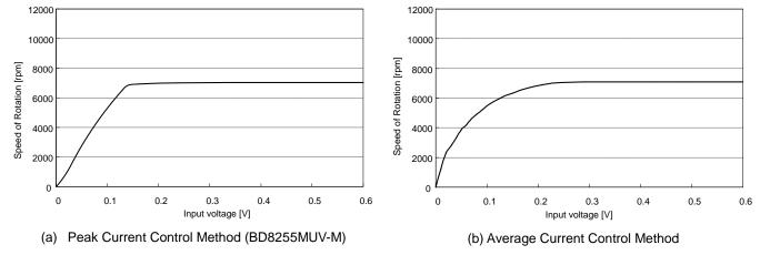
Figure 17. Spindle Driver Input-Output Characteristics
