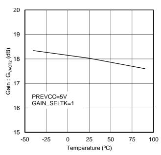
TK Voltage gain 2 (High gain mode)
