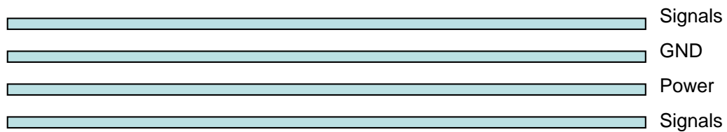
Figure 29: Typical 4-layer PCB construction
