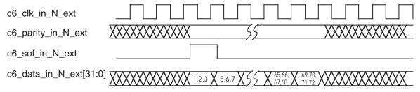
The AC timing specifications for the inbound CSIX port are as follows:
