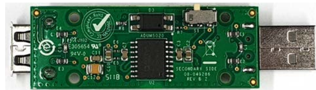
Figure 4. S1 Switch Position for Low Speed Operation
