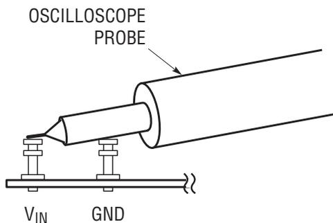
**Figure 2. Proper Input Voltage Ripple Measurement Technique**
