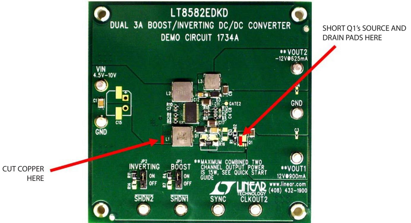
Figure 6. Using Channel 1 Input Disconnect Option (See Text)
