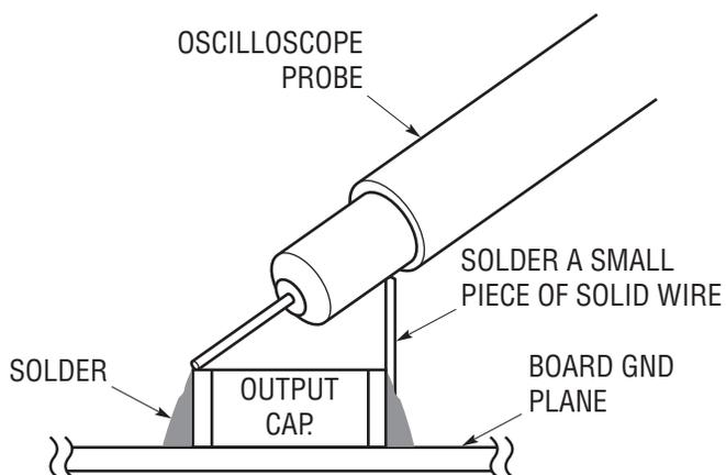
**Figure 3. Proper Output Voltage Ripple Measurement Technique**
