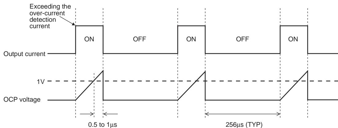
When detecting the output short-circuit state, the short-circuit detection circuit is activated.
