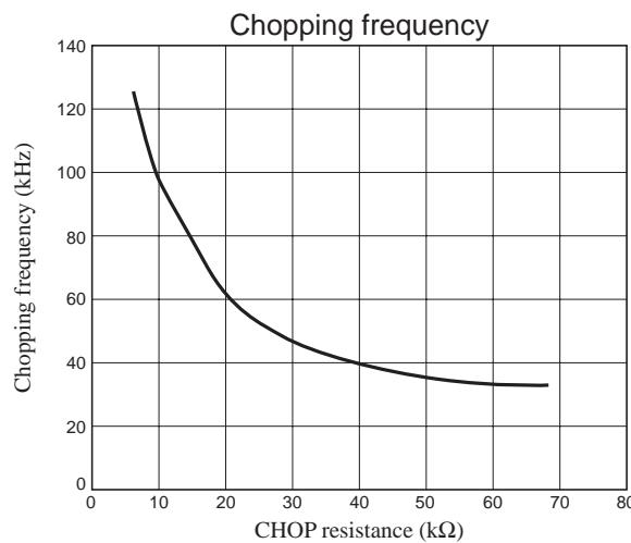
The recommended chopping frequency ranges from 30kHz to 120kHz.
