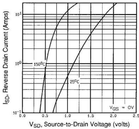
Fig. 7 - Typical Source-Drain Diode Forward Voltage
