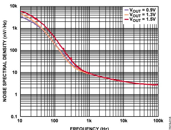
Figure 18. Noise Spectral Density vs. Frequency for Various Output Voltages,
