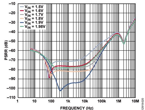
Figure 20. Power Supply Rejection Ratio (PSRR) vs. Frequency for Various  $V_{IN}$ ,
