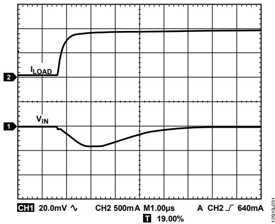
Figure 32. Output Transient Response,  $C_{\text{OUT}} = 47 \mu\text{F}$
