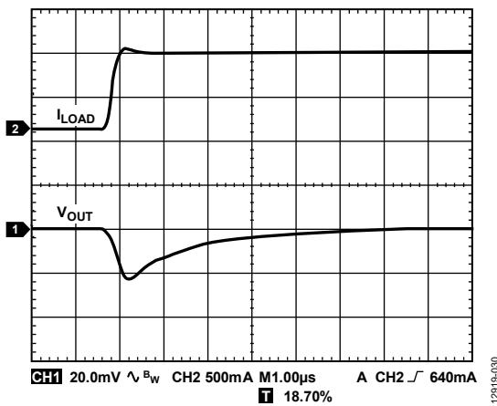
Figure 31. Output Transient Response,  $C_{\text{OUT}} = 10 \mu\text{F}$
