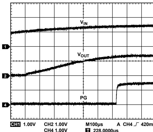
Figure 29. Typical PG Behavior vs.  $V_{OUT}$ ,  $V_{IN}$  Rising ( $V_{OUT} = 1.3$  V)
