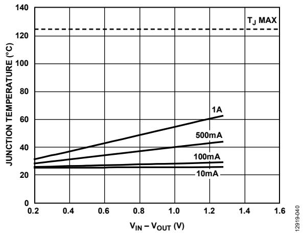
Figure 40. 500 mm<sup>2</sup> of PCB Copper,  $T_B = 25^\circ\text{C}$
