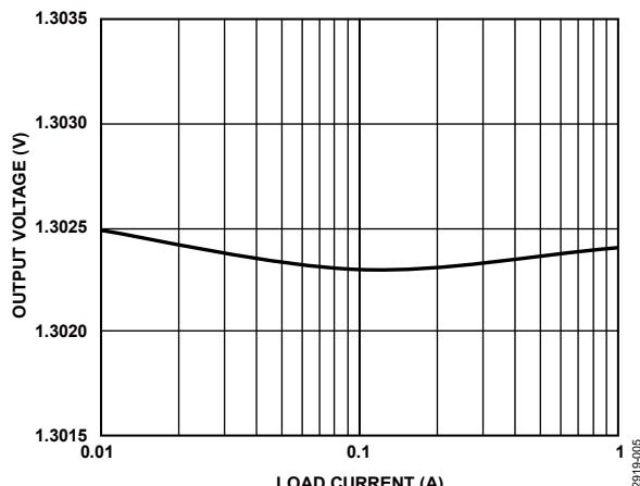
Figure 5. Output Voltage ( $V_{OUT}$ ) vs. Load Current
