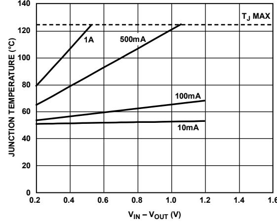
Figure 39. 25 mm<sup>2</sup> of PCB Copper,  $T_A = 50^\circ\text{C}$
