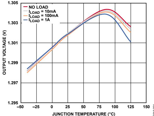
Figure 4. Output Voltage ( $V_{OUT}$ ) vs. Junction Temperature
