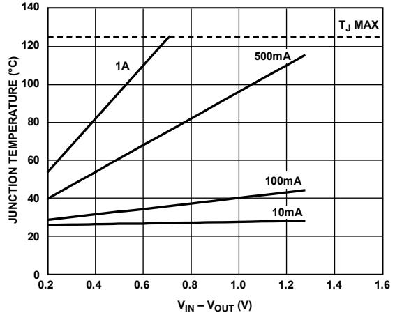
Figure 36. 25 mm<sup>2</sup> of PCB Copper,  $T_A = 25^\circ\text{C}$
