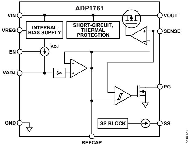
Figure 24. Functional Block Diagram, Adjustable Output
