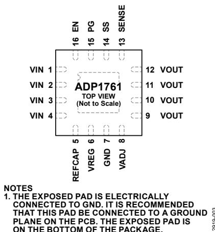
Figure 3. Pin Configuration
