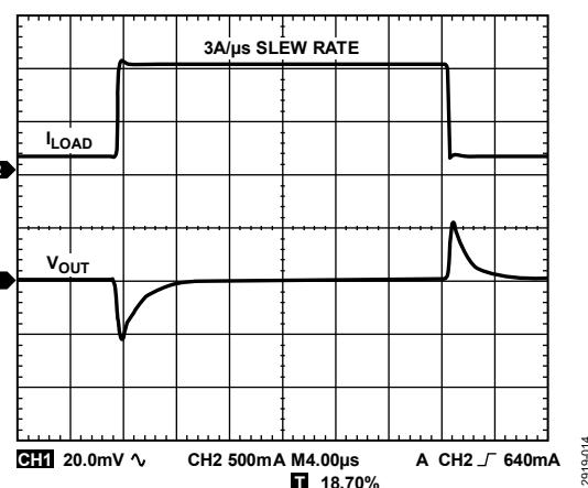
Figure 14. Load Transient Response,  $C_{OUT} = 10 \mu\text{F}$ ,  $V_{IN} = 1.7 \text{ V}$ ,  $V_{OUT} = 1.3 \text{ V}$
