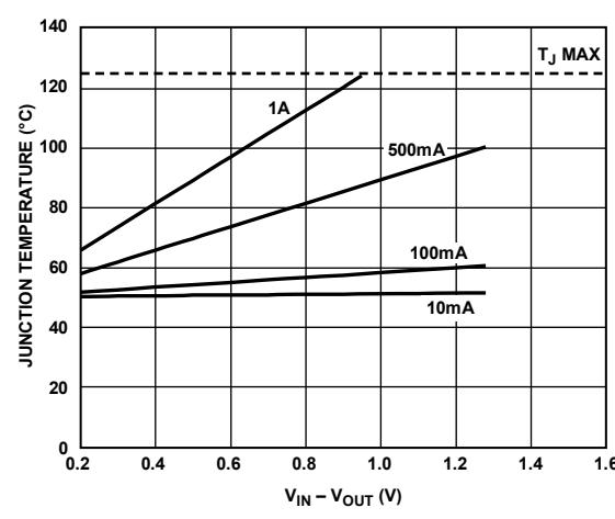
Figure 38. 500 mm<sup>2</sup> of PCB Copper,  $T_A = 50^\circ\text{C}$
