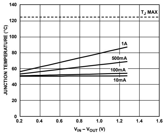
Figure 43. 1000 mm<sup>2</sup> of PCB Copper,  $T_B = 50^\circ\text{C}$
