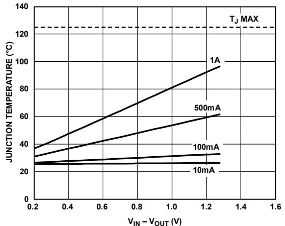
Figure 34. 6400 mm<sup>2</sup> of PCB Copper,  $T_A = 25^\circ\text{C}$
