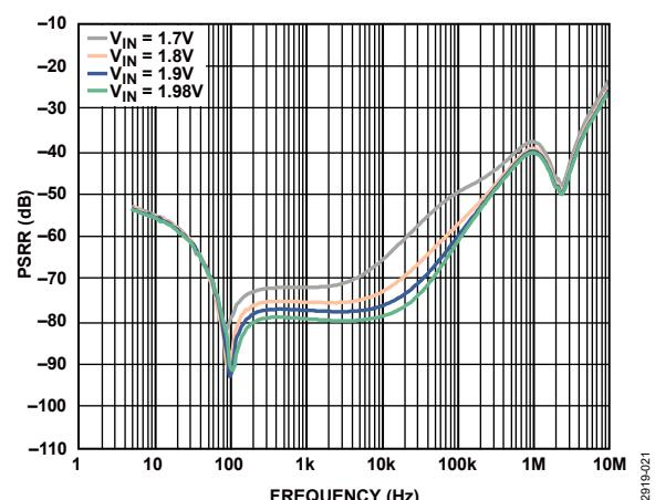
Figure 21. Power Supply Rejection Ratio (PSRR) vs. Frequency for Various  $V_{IN}$ ,
