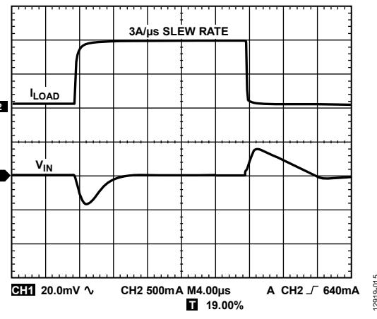
Figure 15. Load Transient Response,  $C_{OUT} = 47 \mu\text{F}$ ,  $V_{IN} = 1.7 \text{ V}$ ,  $V_{OUT} = 1.3 \text{ V}$
