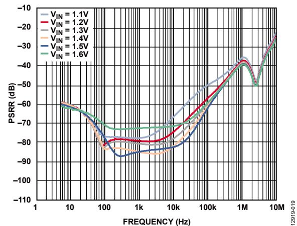
Figure 19. Power Supply Rejection Ratio (PSRR) vs. Frequency for Various  $V_{IN}$ ,
