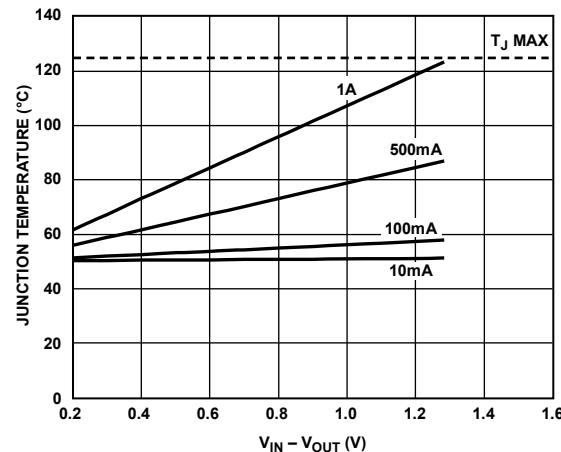
Figure 37. 6400 mm<sup>2</sup> of PCB Copper,  $T_A = 50^\circ\text{C}$
