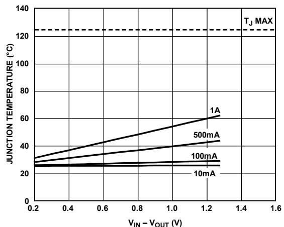
Figure 42. 1000 mm<sup>2</sup> of PCB Copper,  $T_B = 25^\circ\text{C}$
