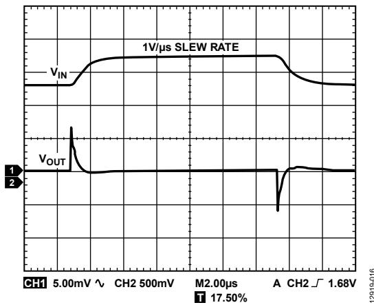
Figure 16. Line Transient Response, Load Current = 1 A,
