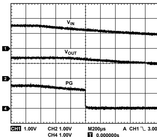
Figure 30. Typical PG Behavior vs.  $V_{OUT}$ ,  $V_{IN}$  Falling ( $V_{OUT} = 1.3$  V)
