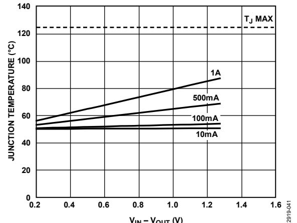
Figure 41. 500 mm<sup>2</sup> of PCB Copper,  $T_B = 50^\circ\text{C}$
