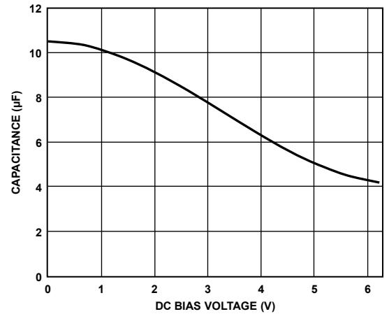
Figure 33. Capacitance vs. DC Bias Voltage
