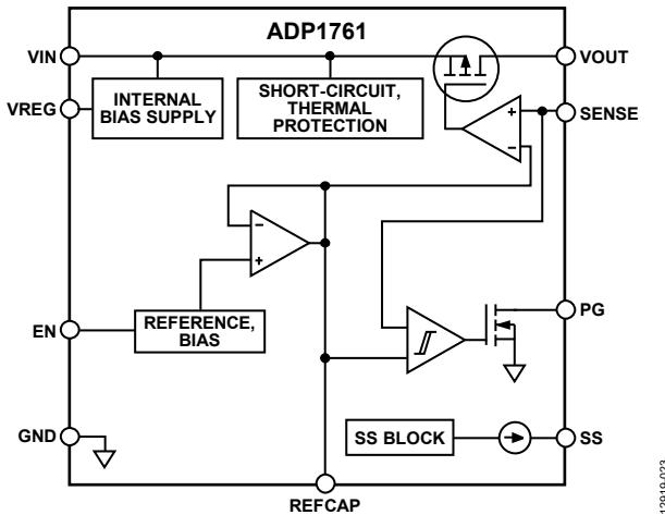
Figure 23. Functional Block Diagram, Fixed Output
