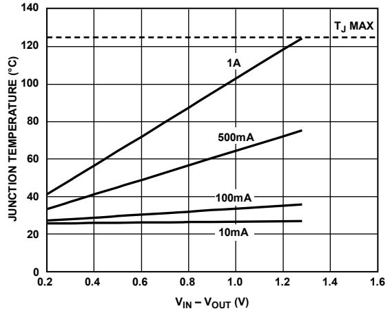
Figure 35. 500 mm<sup>2</sup> of PCB Copper,  $T_A = 25^\circ\text{C}$
