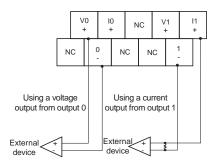
**Note:** The voltage and current output ranges (signals) are set with either the DIP switch or the Configurator settings.
