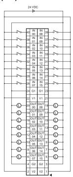
**Screw-less Clamp Terminals with Transistors**
