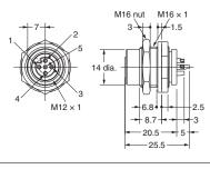
Panel-mounting Connector (Plug) with 0.5 m Cable DCA1-5CNC5M1
