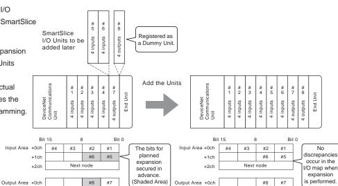
Support for flexible I/O configurations to match the application help downsize the control panel, cut costs, and decrease wiring work.
