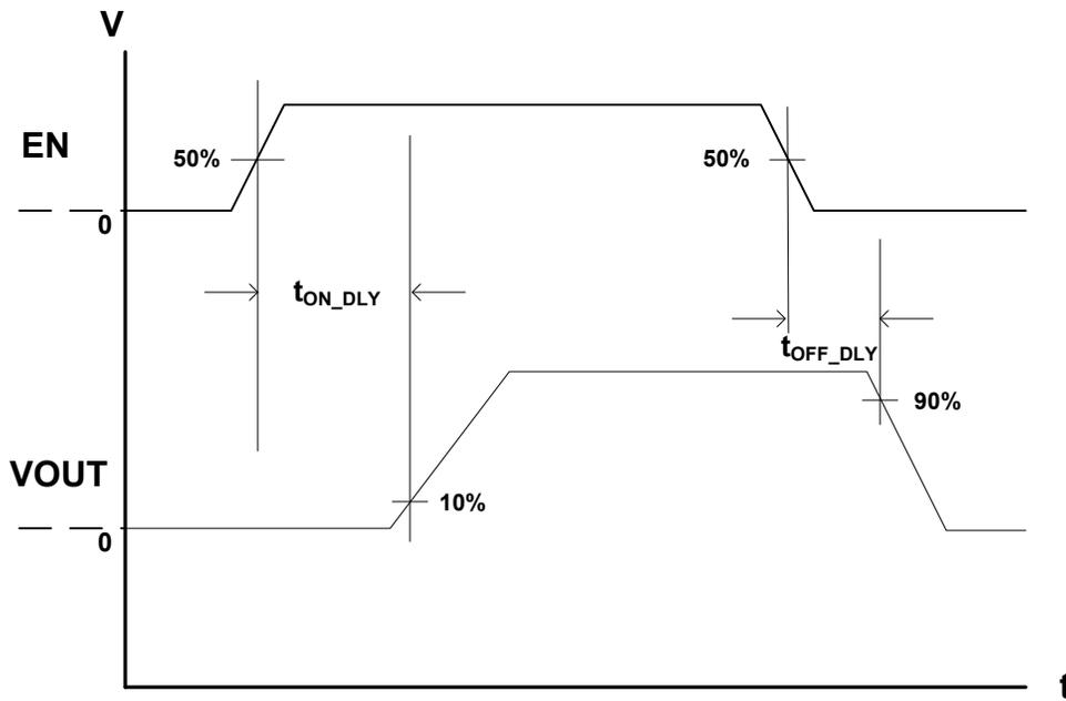
Figure 2. Turn-On/Off Delay
