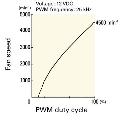
**9BMB24P2K01** With pulse sensor with PWM control function
