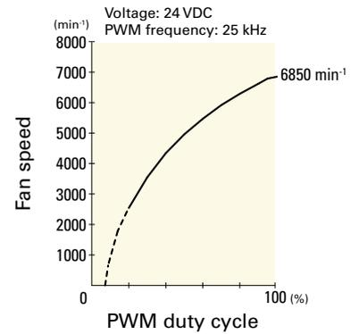
**9BMB24P2G01** With pulse sensor with PWM control function
