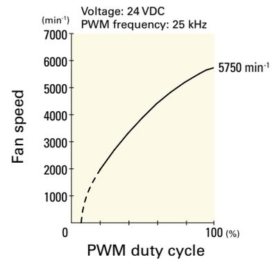
**9BMB24P2S01** With pulse sensor with PWM control function
