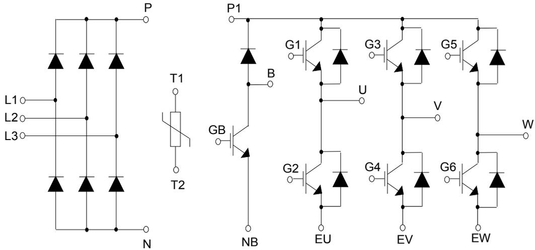
**Figure 22. Package top view with CIB pinout**
