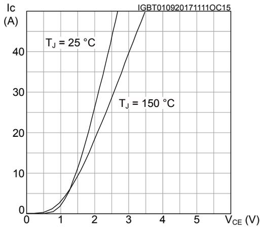
**Figure 4. IGBT output characteristics** ( $T_J = 150\text{ °C}$ , terminal)
