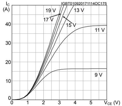
**Figure 5. IGBT transfer characteristics**
