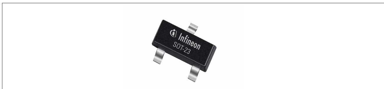
Figure 1-1 Image of TLE4964-4M in the PG-SOT23-3-15 Package
