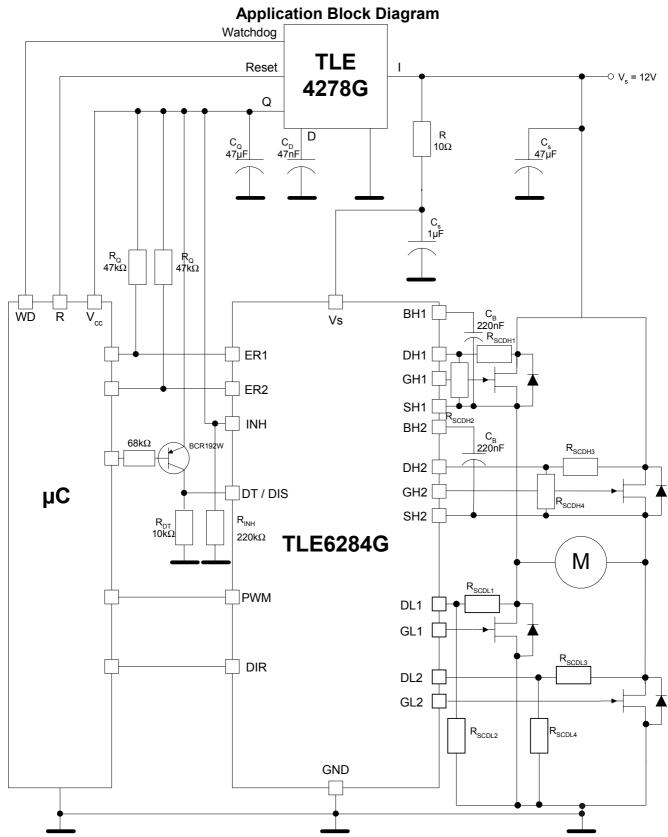
This application block diagram shows one of the possibilities to use this Driver IC. The voltage divider networks accross the 4 MOSFETs (resistors  $R_{\text{SCDxx}}$ ) allow to increase the current limit threshold for Short Circuit protection. The  $R_{\text{SCDLx}}$  resistors also provide a charge path for the bootstrap capacitors. If  $R_{\text{SCDLx}}$  resistors are not used in the application, a 12k Ohm resistor should be introduced between SH1 to GND and SH2 to GND.
