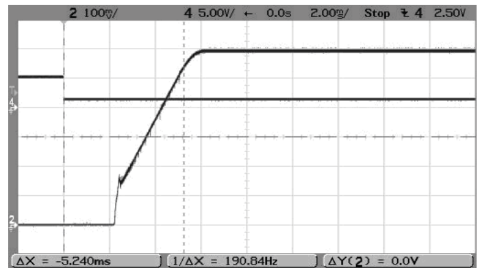
Step Load Transient Response (Vin=5V, Vout=0.6V, Load=0, Iout=3A to 1.5A) Trace 2=Vout, 100 mV/div. Trace 4=Iout, 2.5A/div.
