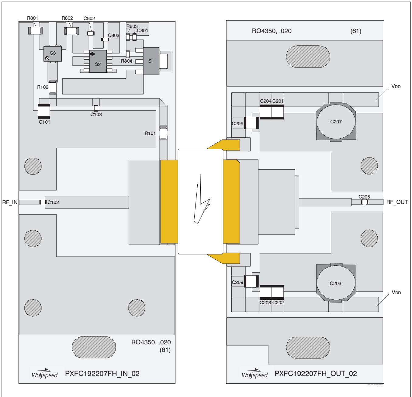
Reference circuit assembly diagram (not to scale)*
