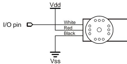
The servo is controlled by pulsing of its signal line. If you are using a Basic Stamp® microcontroller this is done with the 'pulsout' command. Below is PBASIC code that will help you with basic control of a servo. The code below will show center and then rotate the servo to the left and to the right then stop.
