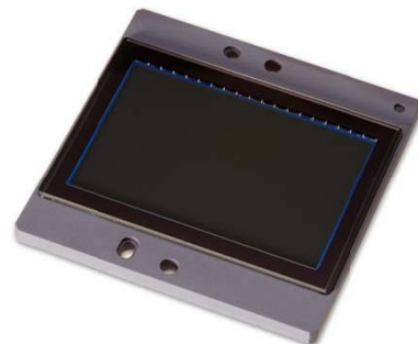
Figure 1. KAI-16000 CCD Image Sensor
