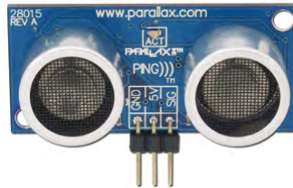
Figure 2-1 The Ping)))™ Ultrasonic Distance Sensor
