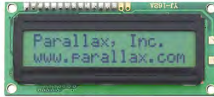
27976 (1) Parallax Serial LCD 2x16, Non-backlit
