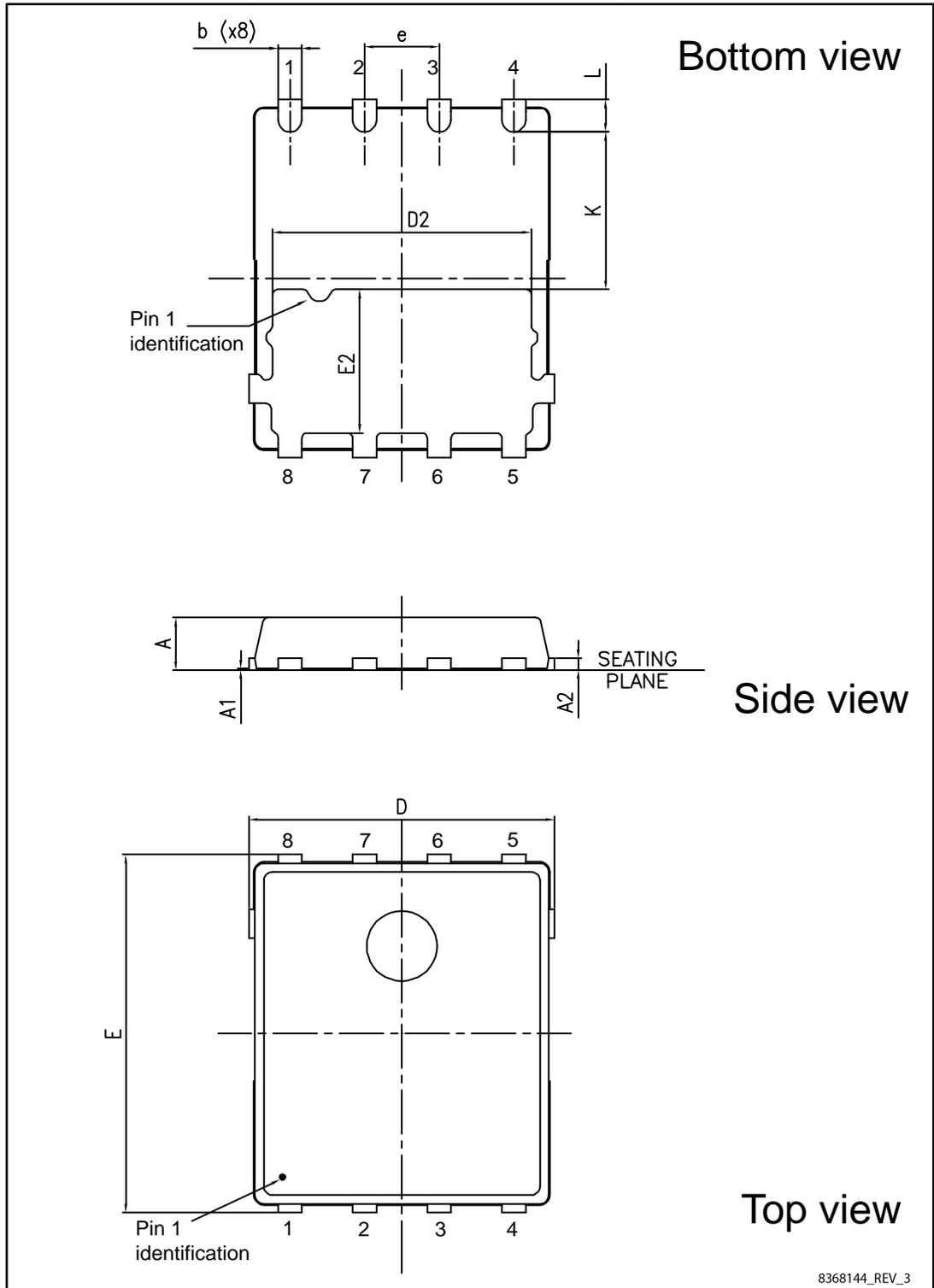
Table 10: PowerFLAT™ 5x6 VHV package mechanical data
