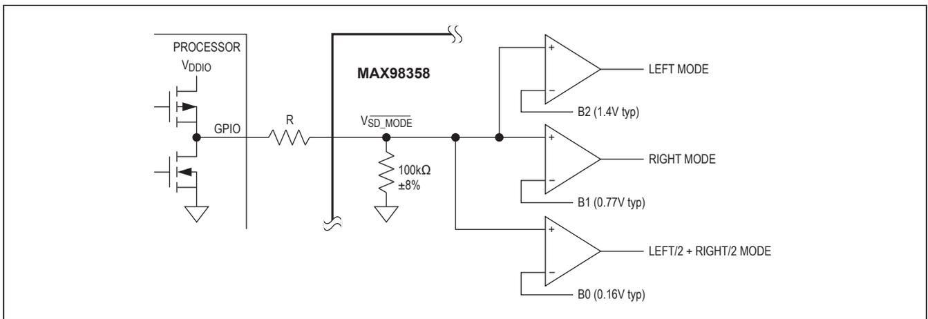
Figure 4.  $\overline{SD\_MODE}$  Resistor Connection Using Push-Pull Driver
