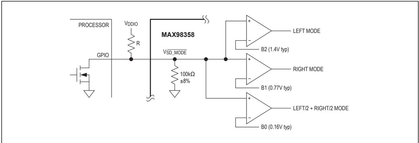
Figure 3.  $\overline{SD\_MODE}$  Resistor Connection Using Open-Drain Driver
