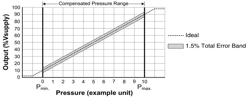
$$\text{Output (V)} = \frac{0.8 \times V_{\text{supply}}}{P_{\text{max.}} - P_{\text{min.}}} \times (\text{Pressure}_{\text{applied}} - P_{\text{min.}}) + 0.10 \times V_{\text{supply}}$$
