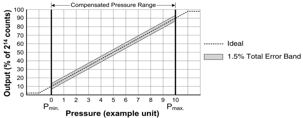
$$\text{Output (\% of } 2^{14} \text{ counts)} = \frac{80\%}{P_{\text{max.}} - P_{\text{min.}}} \times (\text{Pressure}_{\text{applied}} - P_{\text{min.}}) + 10\%$$
