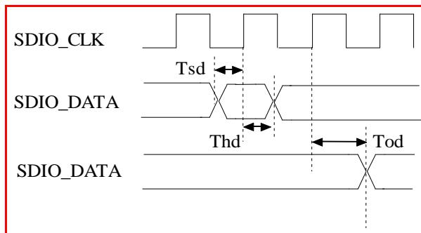
**Figure 6: Interface Timings – SDIO Interface High-speed Mode**
