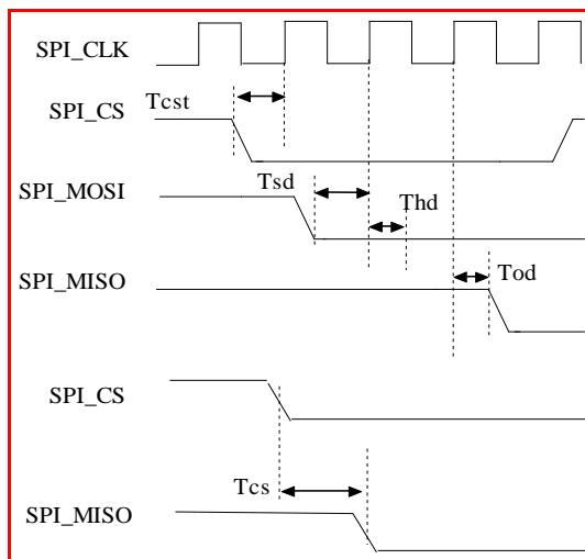
**Figure 9: Interface Timings – SPI Interface High-speed Mode**
