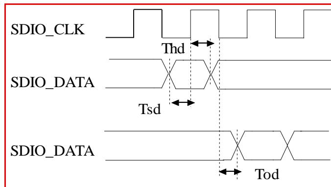
**Figure 5: Interface Timings – SDIO Interface Full-speed Mode**
