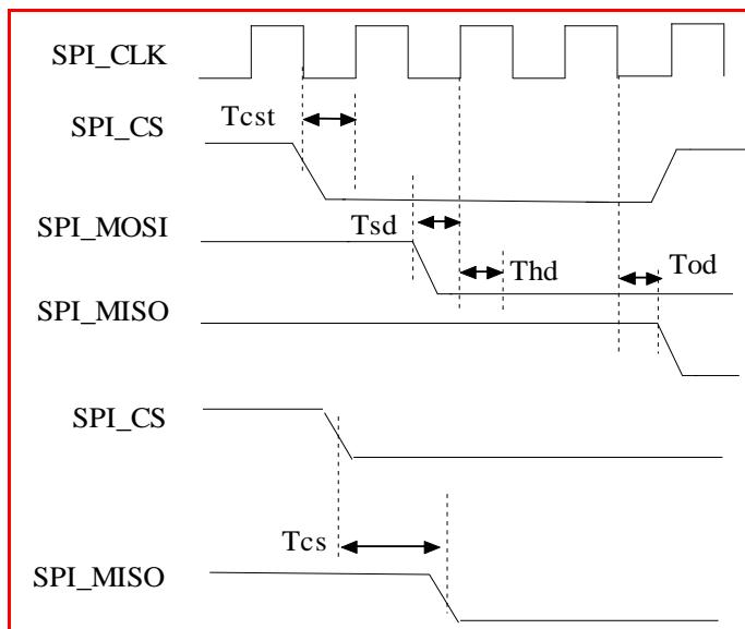
**Figure 8: Interface Timings – SPI Interface Full-speed Mode**
