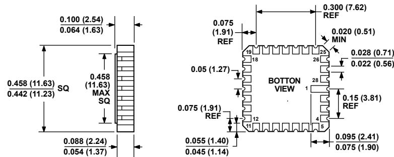
CONTROLLING DIMENSIONS ARE IN INCHES; MILLIMETER DIMENSIONS
