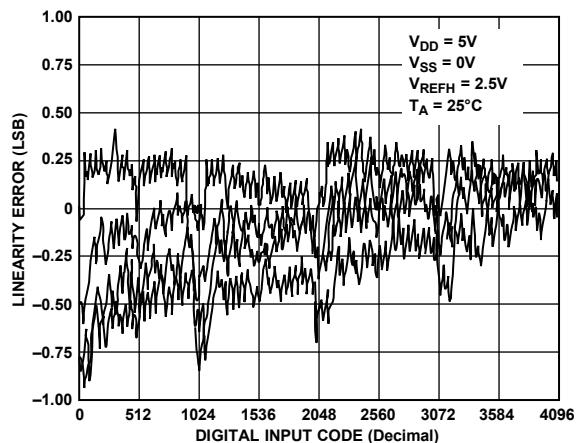
Figure 19. Channel-to-Channel Matching ( $V_{\text{SUPPLY}} = +5 \text{ V}/\text{GND}$ )
