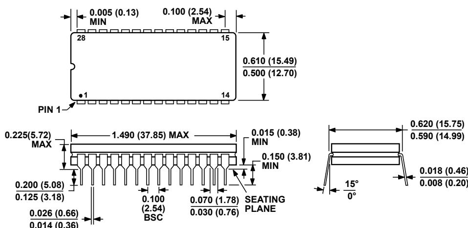
CONTROLLING DIMENSIONS ARE IN INCHES; MILLIMETER DIMENSIONS
