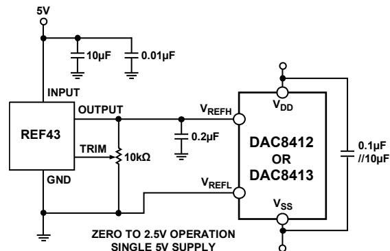
Figure 42.  $+5\ \text{V}$  Single-Supply Operation
