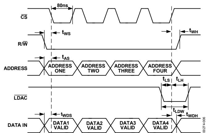
Figure 6. Double-Buffer Mode
