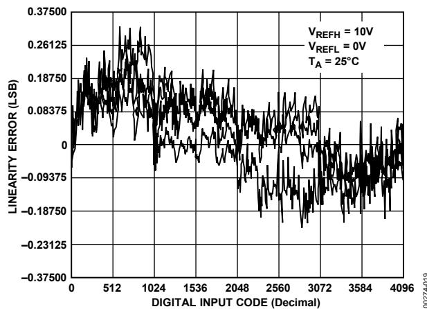
Figure 18. Channel-to-Channel Matching ( $V_{\text{SUPPLY}} = \pm 15 \text{ V}$ )
