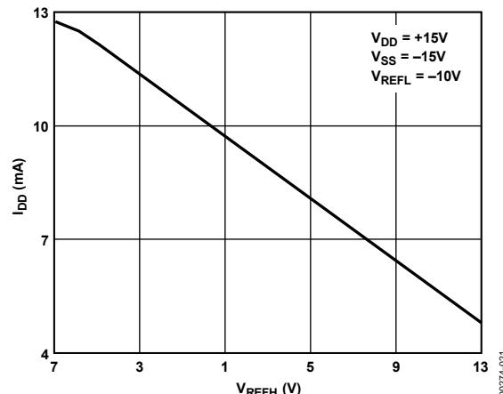
Figure 20.  $I_{\text{DD}}$  vs.  $V_{\text{REFH}}$  (All DACs High)
