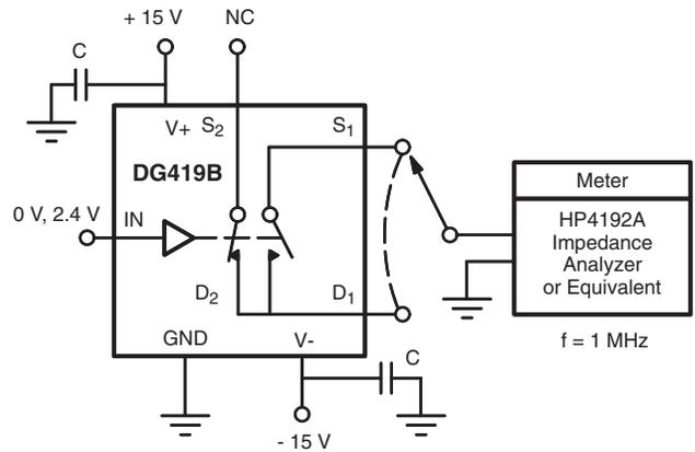
**Figure 9. Source/Drain Capacitances**
