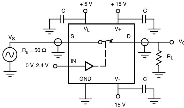
**Figure 8. Insertion Loss**
