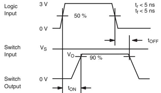
Note: Logic input waveform is inverted for switches that have the opposite logic sense.
