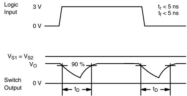
Figure 3. Break-Before-Make (DG419B)
