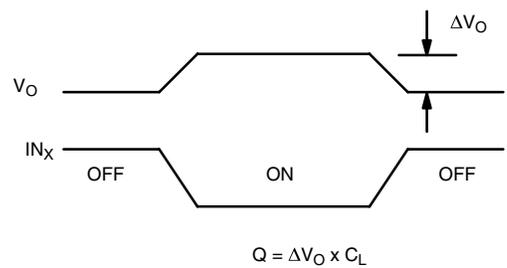
Figure 5. Charge Injection
