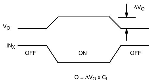
Figure 5. Charge Injection
