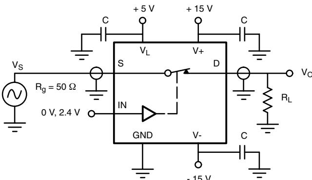
**Figure 8. Insertion Loss**
