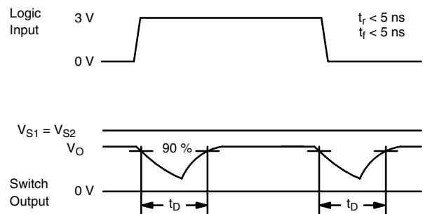
Figure 3. Break-Before-Make (DG419B)
