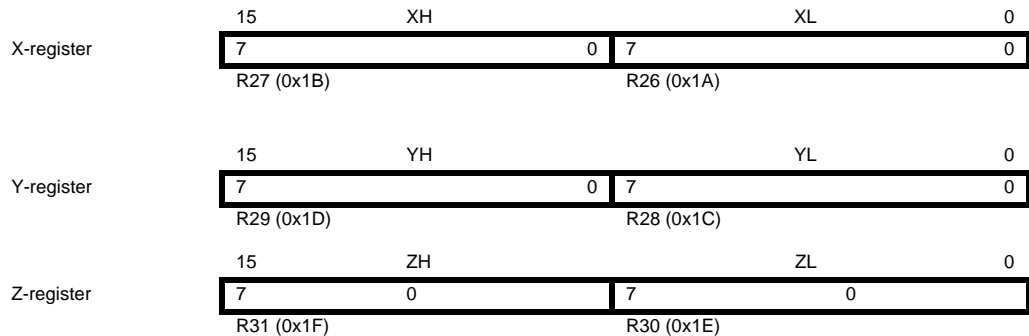
Figure 6-3. The X-, Y-, and Z-registers
