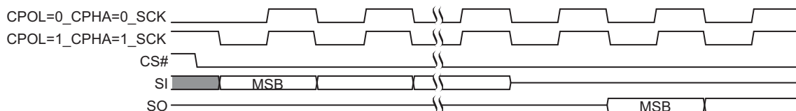
Figure 4. SPI SDR Modes Supported
