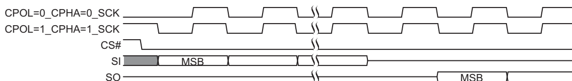
Figure 4. SPI SDR Modes Supported
