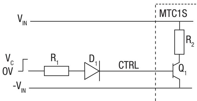
$D_1$  (e.g. 1N4001) is required to provide high impedance when the signal is low. From the MTC1 specification, the drive current to operate this function is recommended to be 3mA to 8mA, and hence the value of  $R_1$  can be derived as follows:
