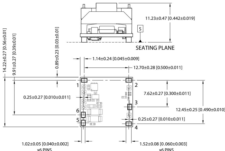
All dimensions in mm(inches). Controlling dimension is mm. Tolerances (unless otherwise stated)  $\pm 0.10(0.004)$ .
