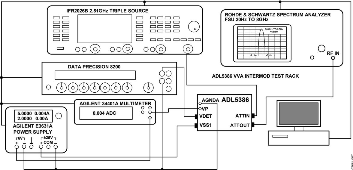
Figure 57. ADL5386 Characterization Board VVA Intermodulation Test Setup
