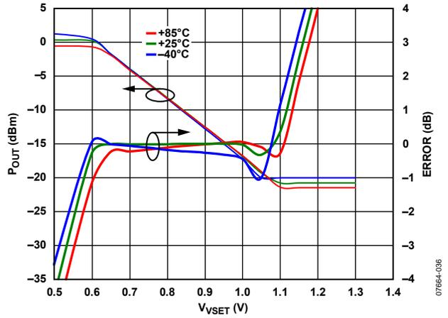
Figure 36.  $P_{OUT}$  and Error vs.  $V_{VSET}$  at 1450 MHz
