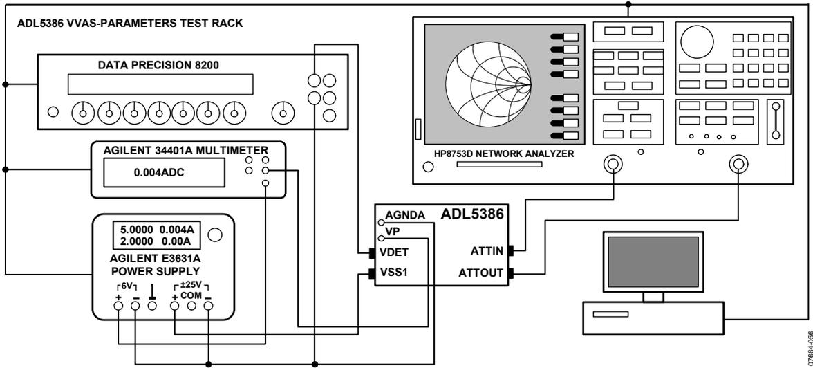
Figure 56. ADL5386 Characterization Board VVA S-Parameters Test Setup
