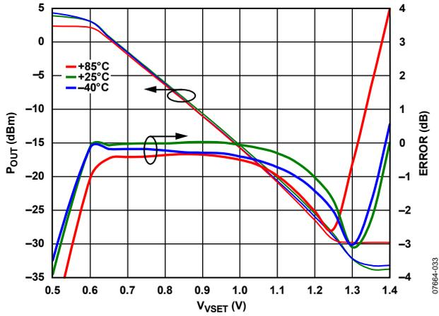
Figure 33.  $P_{OUT}$  and Error vs.  $V_{VSET}$  at 140 MHz
