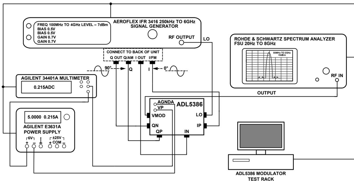
Figure 54. ADL5386 Characterization Board SSB Test Setup
