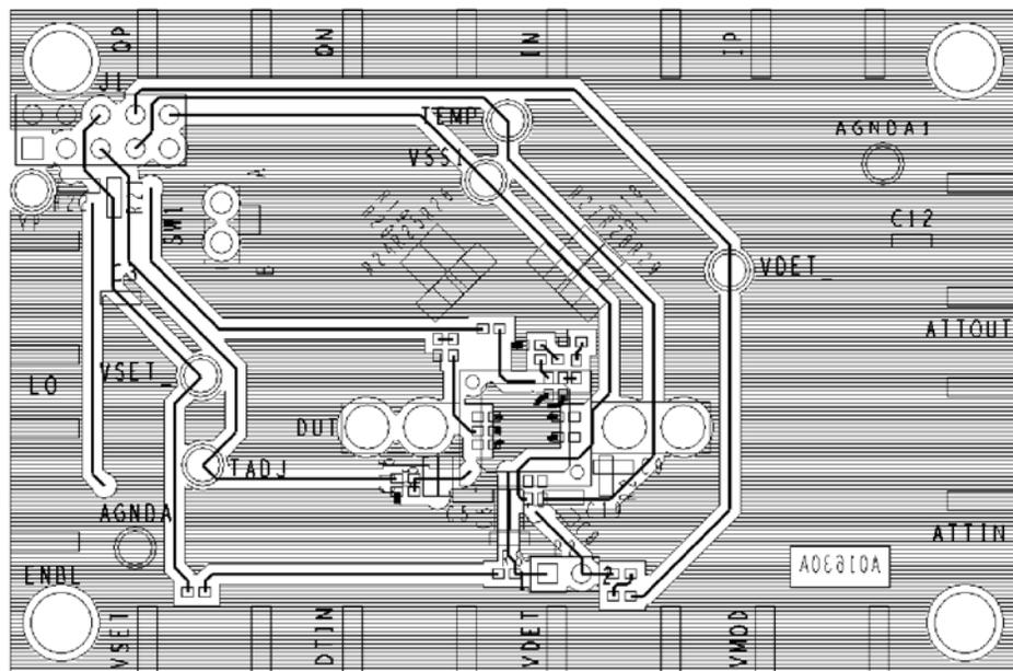
Figure 53. Layout of the Evaluation Board, Bottom Layer
