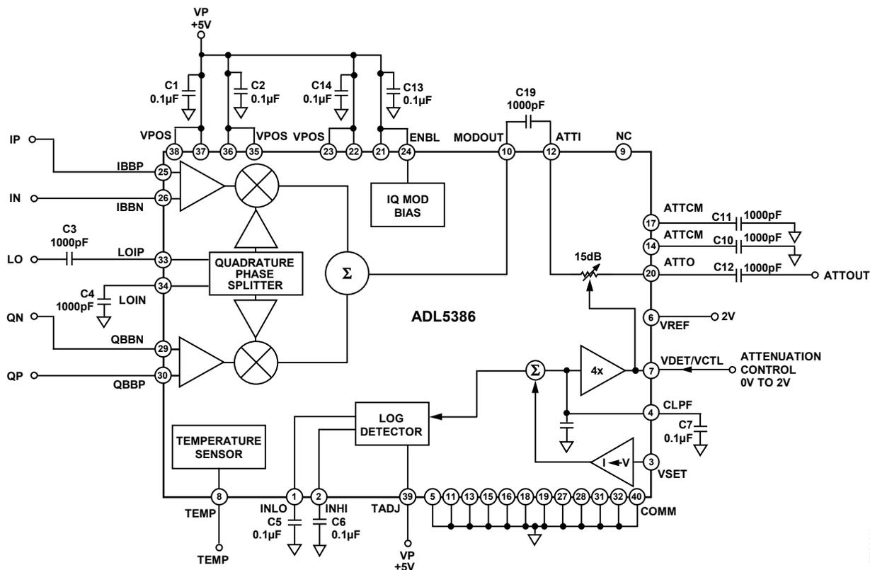
Figure 41. Basic Connections for Open-Loop Power Control Mode
