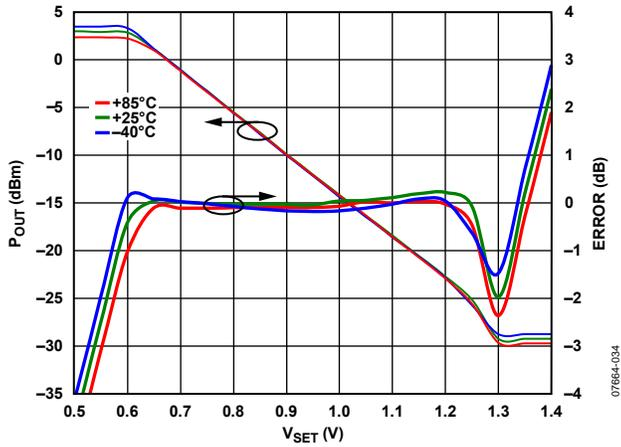
Figure 34.  $P_{OUT}$  and Error vs.  $V_{VSET}$  at 350 MHz
