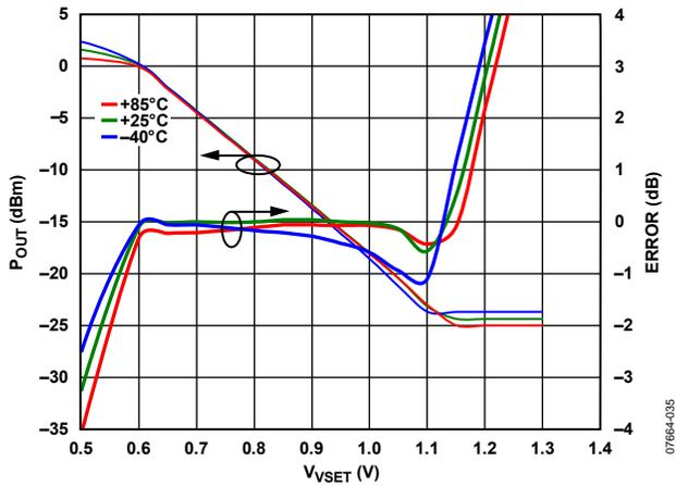
Figure 35.  $P_{OUT}$  and Error vs.  $V_{VSET}$  at 860 MHz
