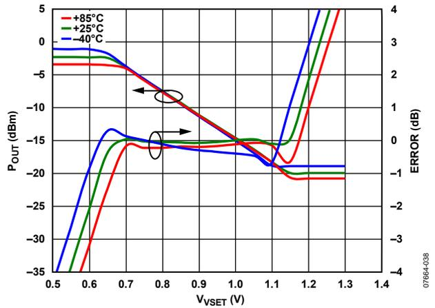
Figure 38.  $P_{OUT}$  and Error vs.  $V_{VSET}$  at 2150 MHz
