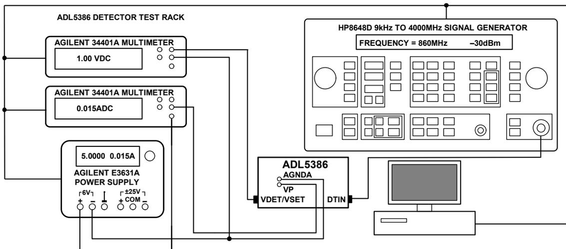
Figure 55. ADL5386 Characterization Board Detector Test Setup
