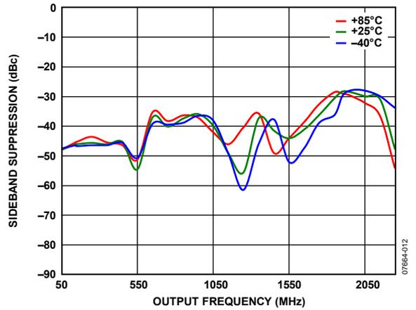
Figure 12. Sideband Suppression vs. Output Frequency and Temperature
