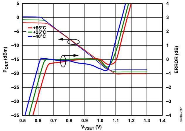
Figure 37.  $P_{OUT}$  and Error vs.  $V_{VSET}$  at 1900 MHz
