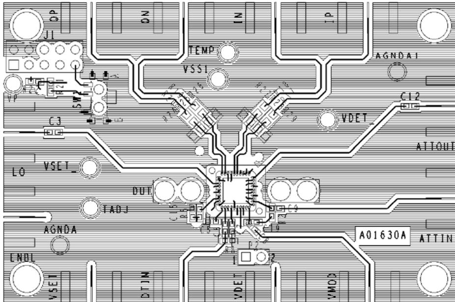
Figure 52. Layout of the Evaluation Board, Top Layer
