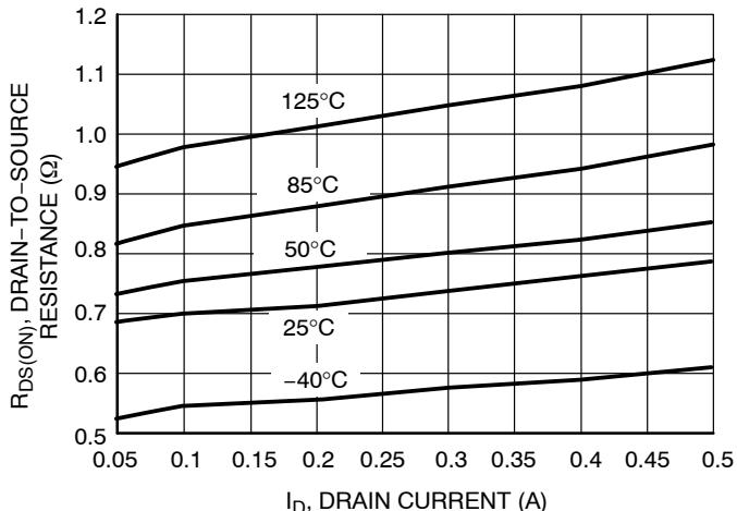
Figure 8. On-Resistance vs. Drain Current and Temperature
