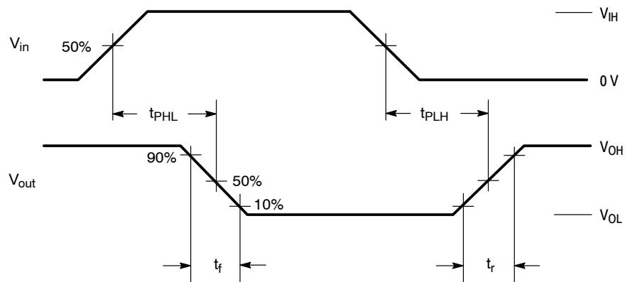
Figure 1. Switching Waveforms
