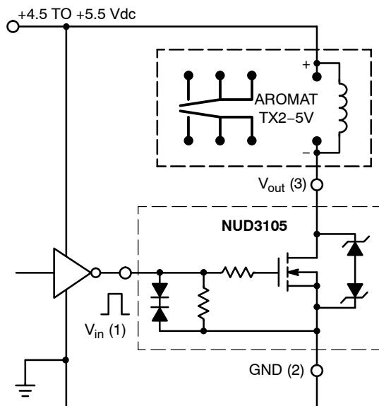
Figure 13. A 140 mW, 5.0 V Relay with TTL Interface
