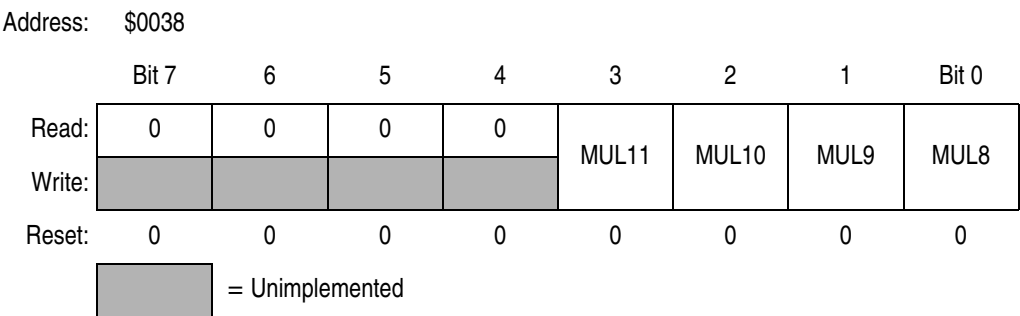
Figure 8-6. PLL Multiplier Select Register High (PMSH)
