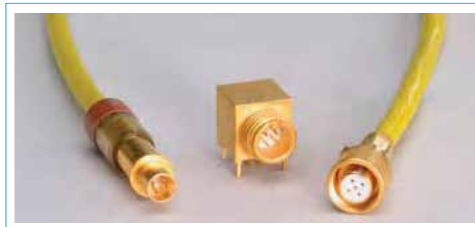
90° Quadrax Receptacle and Plug Transition Adapter
