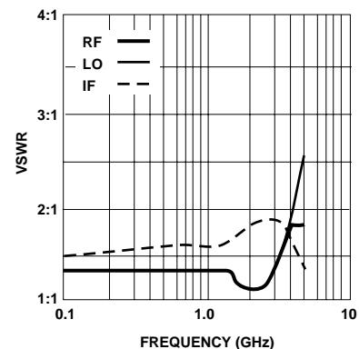
**Figure 4. RF, LO and IF Port VSWR vs. Frequency.**
