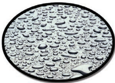
Solder beads off the porcelain coating like water on a freshly waxed car
