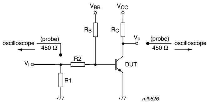
I<sub>C</sub> = 0.5 A; I<sub>Bon</sub> = 25 mA; I<sub>Boff</sub> = -25 mA; R<sub>1</sub> = open; R<sub>2</sub> = 100 Ω; R<sub>B</sub> = 300 Ω; R<sub>C</sub> = 20 Ω
