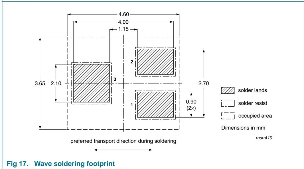
**Fig 17. Wave soldering footprint**
