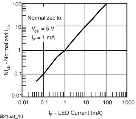
Fig. 10 - Normalized Collector Base Photocurrent vs. LED Current
