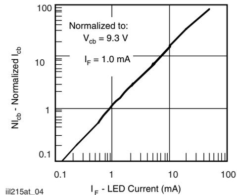
Fig. 4 - Normalized Collector Base Photocurrent vs. LED Current
