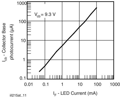
Fig. 11 - Collector Base Photocurrent vs. LED Current
