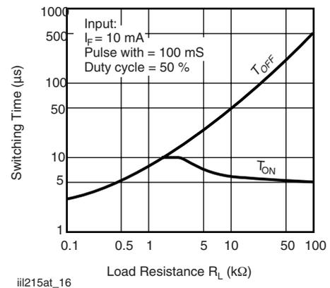
Fig. 16 - Typical Switching Times vs. Load Resistance
