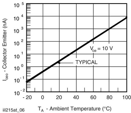
Fig. 6 - Collector Emitter Leakage Current vs. Temperature
