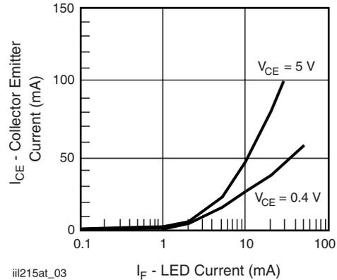
Fig. 3 - Collector Emitter Current vs. LED Current
