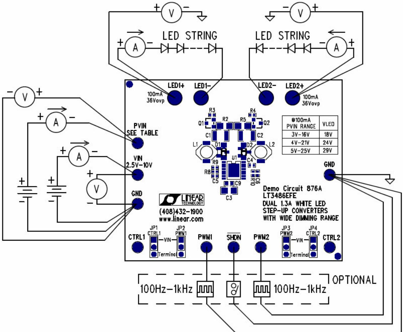
Figure 3. Proper Measurement Equipment Setup
