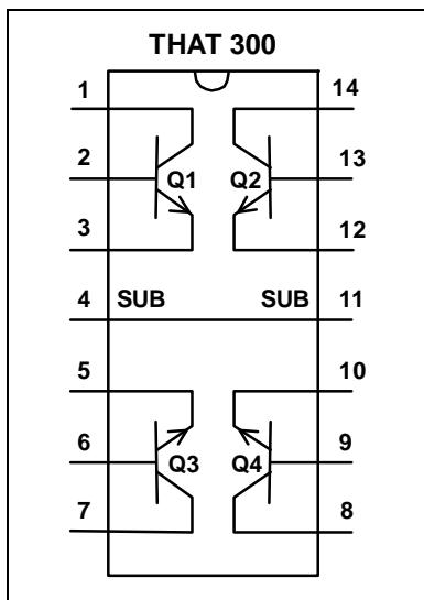
Figure 1. 300 Pinout
