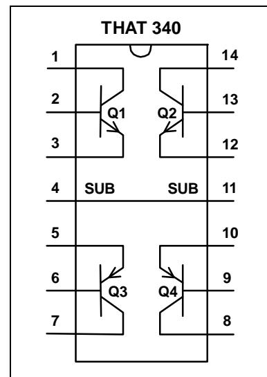
Figure 3. 340 Pinout
