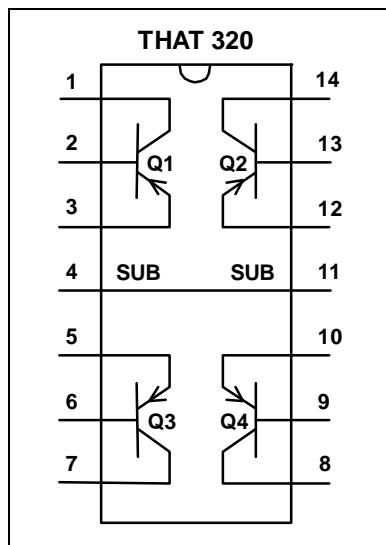
Figure 2. 320 Pinout
