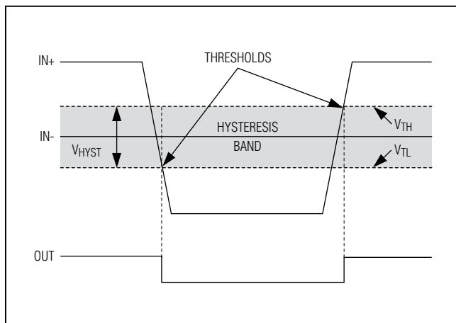
Figure 1. Threshold Hysteresis Band (Not to Scale)
