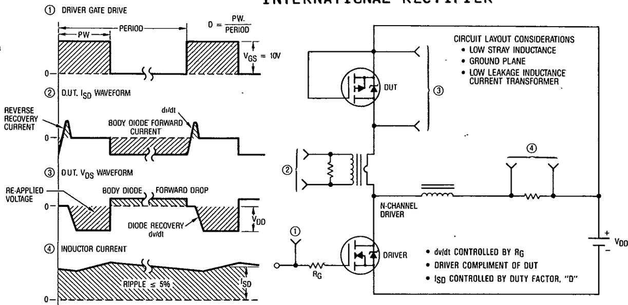
Fig. 17 — Peak Diode Recovery  $dv/dt$  Test Circuit
