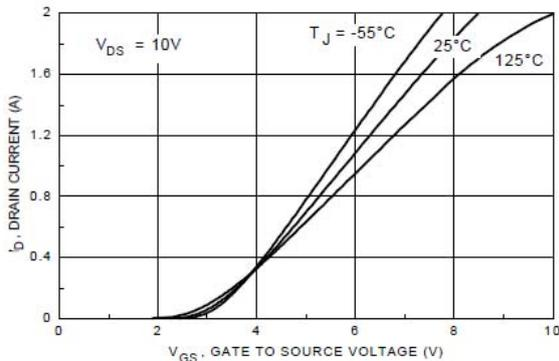
Figure 5. Transfer Characteristics.
