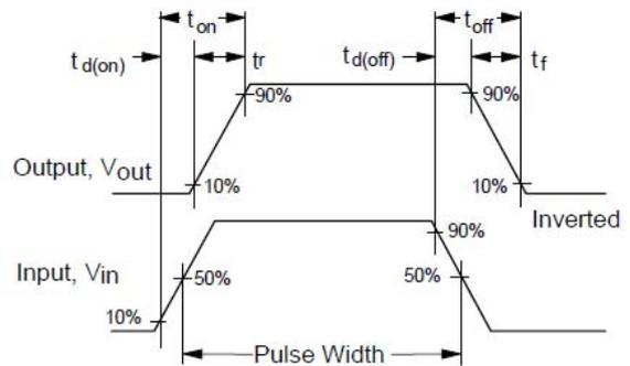
**Figure 12. Switching Waveforms.**
