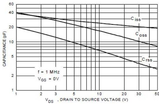
**Figure 9. Capacitance Characteristics.**
