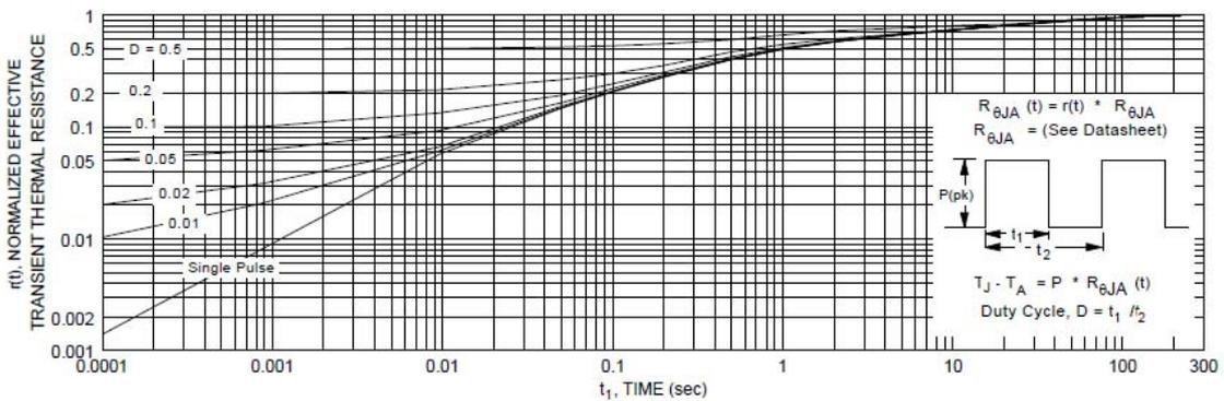
Figure 16. SOT-23, MMBF170 Transient Thermal Response Curve.
