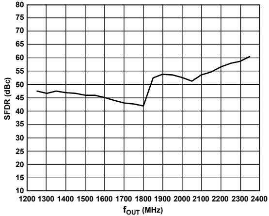
Figure 52. SFDR vs. f_{OUT} in Mix Mode, f_{DAC} = 2.4 GHz, Full-Scale Current = 20 mA (Second Nyquist Zone Performance)
