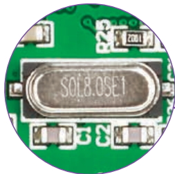
Figure 5-1: Crystal oscillator module (X1)
