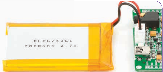
Figure 1-2: Connecting Li-Polymer battery
