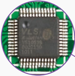
Figure 8-1: On-board VS1053 MP3 codec
