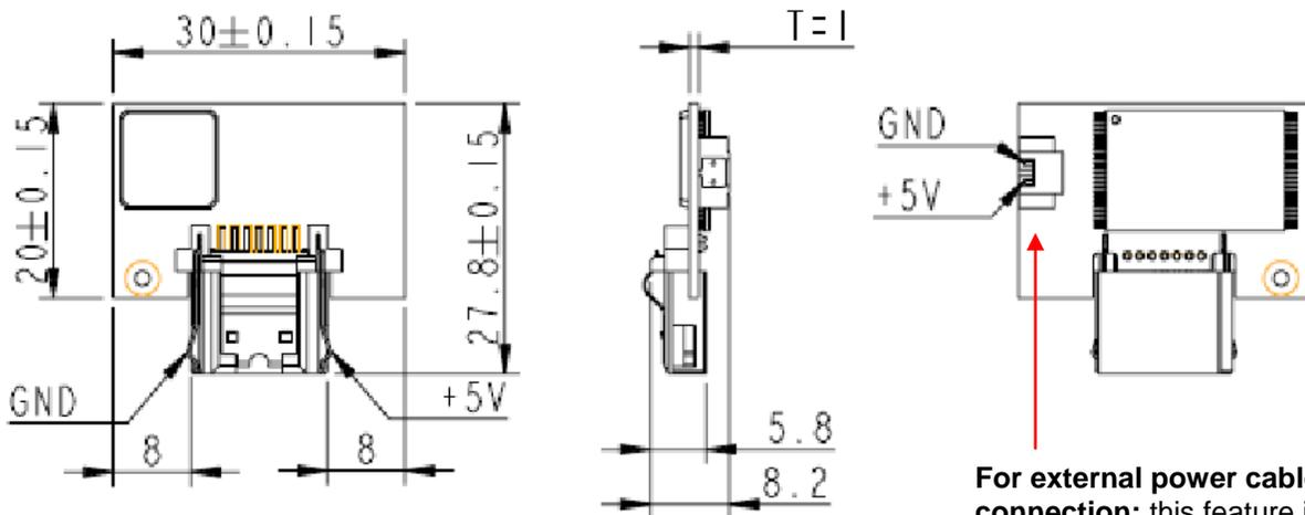
**For external power cable connection:** this feature is available as an option for Standard Type.
