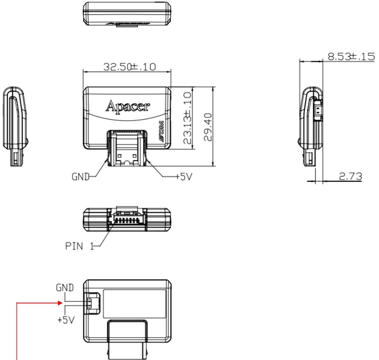
**For external power cable connection:** this feature is available as an option for Standard Type.
