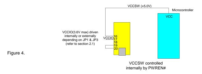
Figure 4 shows how to connect the switched +5.0V power to external logic circuits. The internal "soft-start" circuit on the DLP-2232H accommodates designs that draw more than 100mA at power up.
