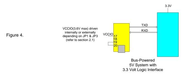
Figure 4 shows how to configure the DLP-2232H to interface with a 3.3V logic device via the ASYNC serial mode. In this example, the target electronics provide the 3.3 volts to power the microcontroller.
