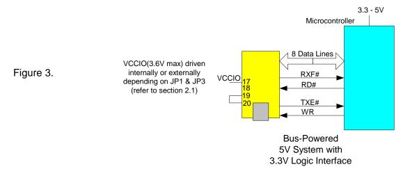
Figure 3 shows how to configure the DLP-2232H to interface with a microcontroller via the parallel 245 FIFO interface mode. In this example, the target electronics can operate at from 3.3 - 5 volts since the DLP-2232H interface I/O pins are 5 volt tolerant.
