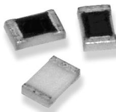
Precious metal terminations are screen printed onto a ceramic base and fired. The resistive element is screen printed and fired and the passivation layer added. The pre-scribed tile is broken into strips, the end plating is fired on and the strips broken into individual components. Final termination is made by electroplating.
